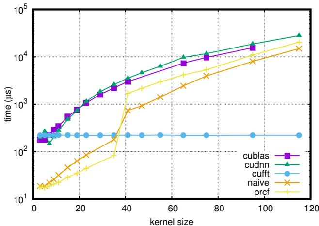
Fig. 2: Execution time in single precision
