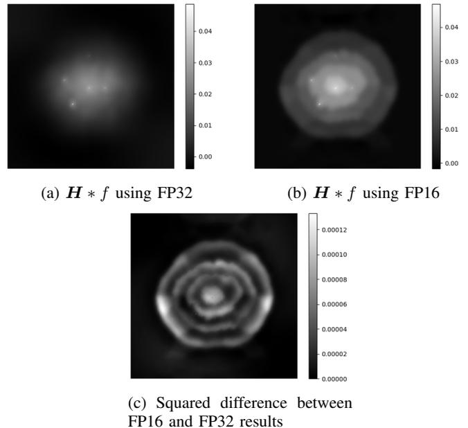
Fig. 8: Convolution errors with our dataset
